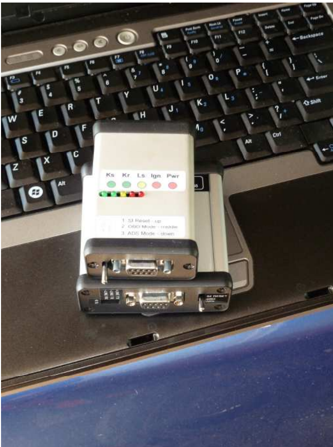
Connection to either the round 20 pin diagnostic port under the hood, or to a 16 pin OBD port under the dash of later cars is a snap .
