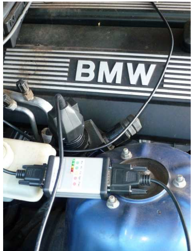
Connection to either the round 20 pin diagnostic port under the hood, or to a 16 pin OBD port under the dash of later cars is a snap .
