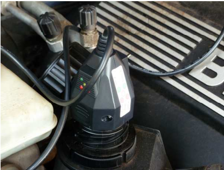
Rv8flyboy's round 20 pin integrated interface and serial cable connects directly between the round 20 pin diagnostic port under the hood of your car and your computer's serial port.
